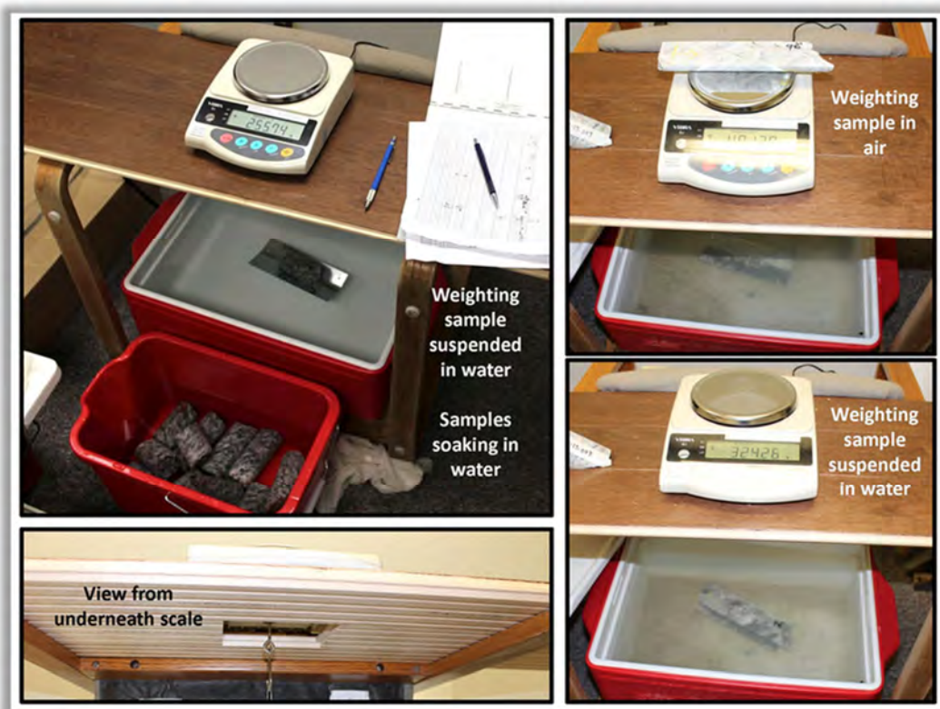
Figure 14.1 Specific Gravity Station
